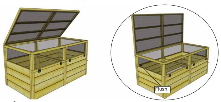
**6.** To complete Trellis/Lid installation, lift lid up and position in an upright position. You will have to hold in this position until Trellis/Lid arms are installed so an assistant would be helpful.
