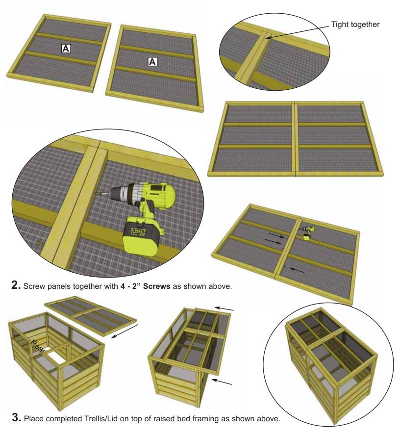
Important - If Raised Bed is not square and level, Trellis/Lid may not fit and align correctly. Before positioning, measure and align bed framing as square as possible.
