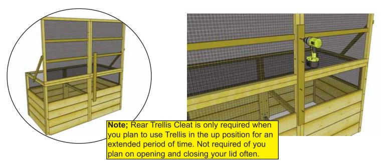
**10.** If required, locate **Rear Trellis Cleat (D)**. Center on 6x3 Raised Bed center framing and Trellis/Lid panel framing. Attach with **4 - 2" screws** slighly offset from the center. At the end of your gardening season, carefully remove screws from cleat and store to use again for the next year.
