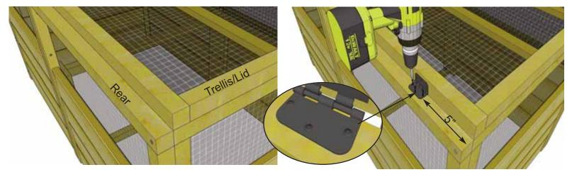
**4.** With Trellis/Lid evenly positioned on raised bed framing, locate **4 Black Plastic Hinges - Part B** and **24 - 3/4" Black Screws.** Align 1st hinge with counter sunk holes facing up. Position hinge approx. 5" from end. Attach to top framing of 6x3 raised bed with **3 - 3/4" Black Screws** per hinge. Pre-drill shallow hinge holes first with 1/8" drill bit to prevent wood from splitting. Do not over screw with cordless screw gun!
