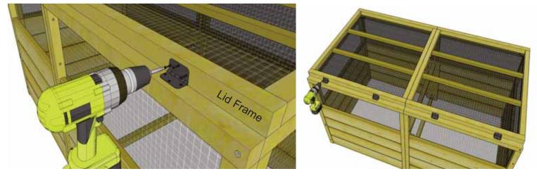
**5.** Complete attachment of 1st hinge by screwing **3 - 3/4**" **Black Screws** into the lid framing as shown above. Evenly space remaining hinges and attach as described previously.
