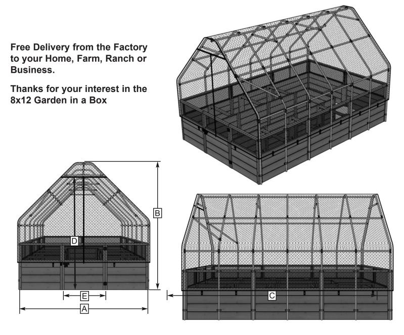
Product Specifications:A:Width = 95"B:Height = 91"C:Depth = 140"D&E:Doorway = 78"h x 30"w\* Framing Material - 1" diameter steel tubing powder coated black.Weighted black.
