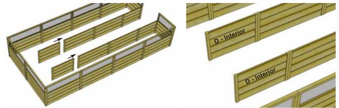
**12.** Align and attach final side **Interior Panels (Part D)** as per **Step 10**. Angle screw panels together with **3 - 2 1/2" Screws** from the inside.
