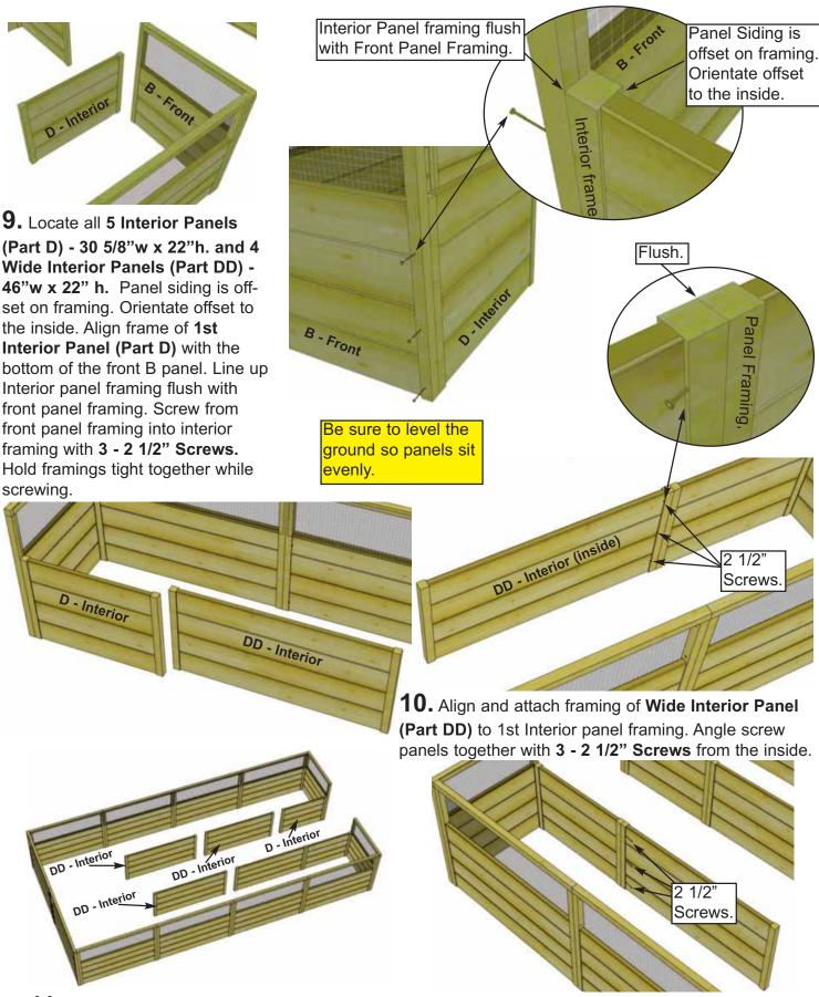
**11.** Align and attach framing of **(Part D)** and **(Part DD)** Panels as per **Steps 9 & 10**. Angle screw panels together with **3 - 2 1/2" Screws** from the inside.
