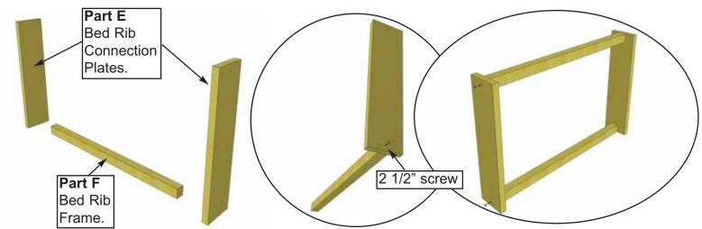
13. To complete rib assembly, locate all 10 Bed Rib Connection Plates (Part E) - 1" x 5 1/2" x 20".
