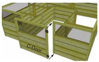
**19.** Locate **Door Panel (Part C) - 30 5/8" w x 33 1/2" h)** and position on flat surface screen down. Attach both hinges to door panel with **3 - 3/4" Black Headed Screws** per hinge. Space hinges evenly on door frame. Pre-drill shallow hole first to prevent wood from splitting.
